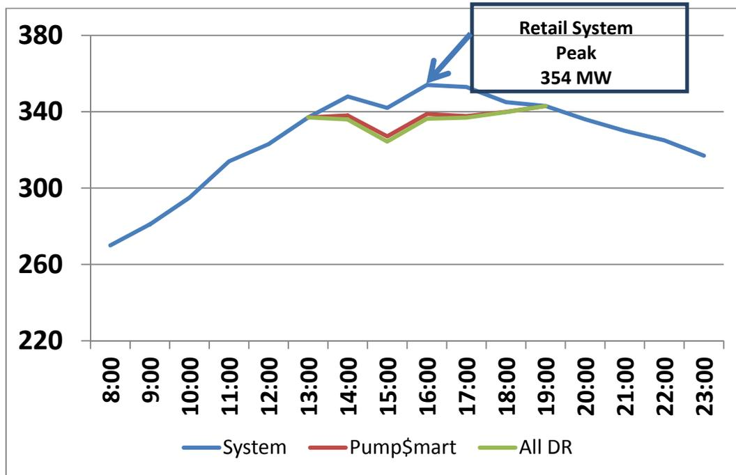
As illustrated by Chart I above, the DR capability at the time of the system peak and during the time of typical interruption events (phased in and out from 2 PM until 7 PM) could have significantly reduced the peak. During the peak hour, over 88.4% (15.2 MW) of the subscribed capacity in the Pump\$mart program was available for dispatch.
