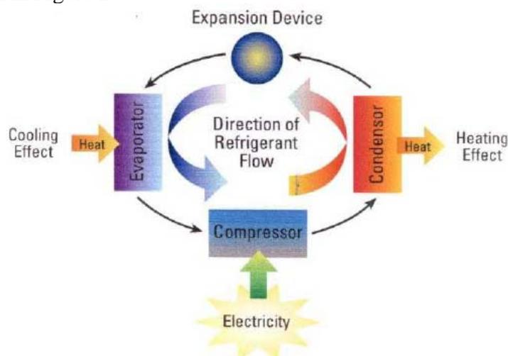
**Figure 2.** Operation of a Heat Pump.<sup>9</sup> Liquid refrigerant at high pressure is forced through an expansion valve into a low-pressure evaporator. The liquid evaporates, absorbing heat from the surrounding area. The gaseous refrigerant is then compressed by an electric compressor. At high pressure, the refrigerant condenses back into a liquid, rejecting heat into its surroundings.
