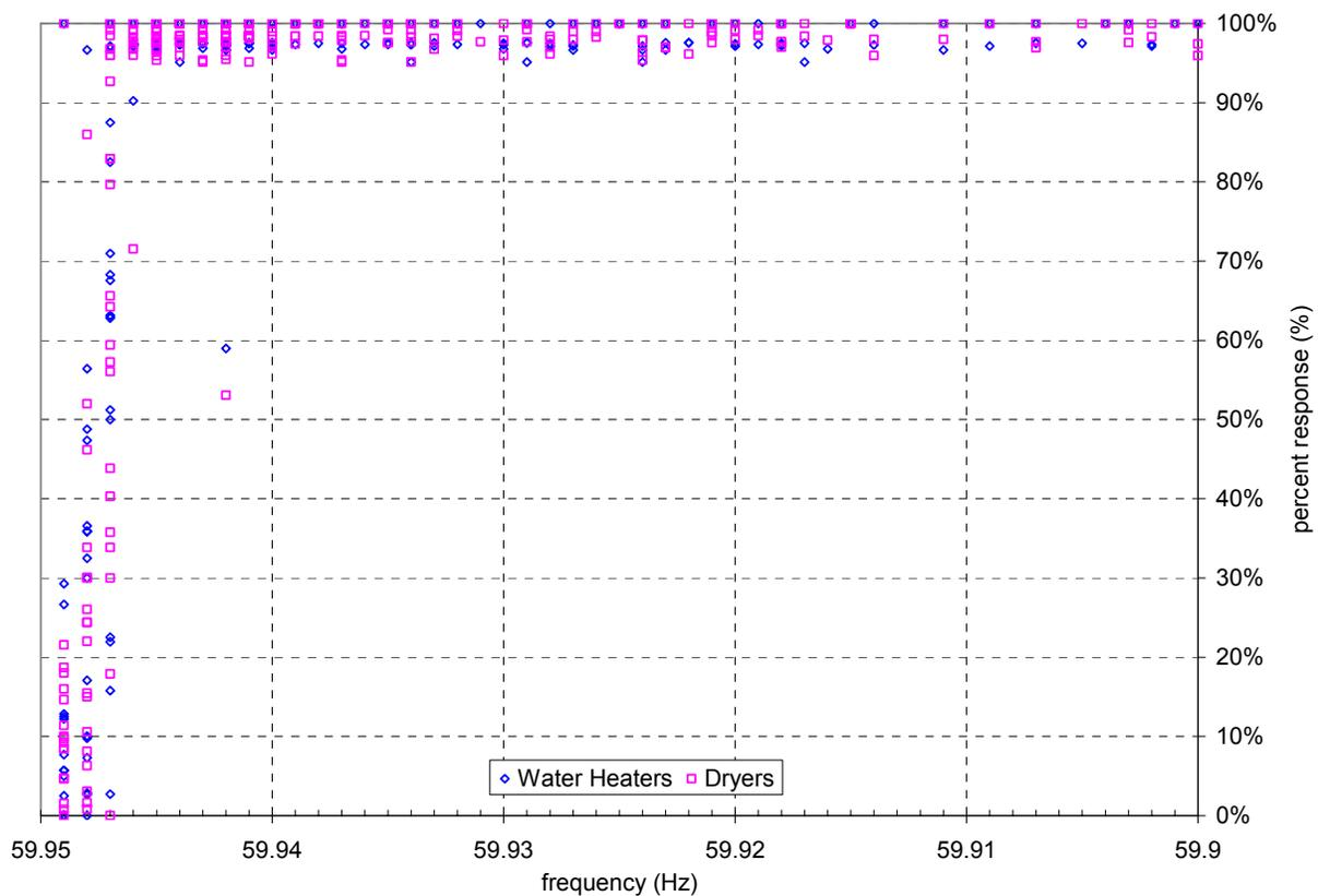
**Figure 7.** Percentage of GFA Controllers Successfully Detecting Events versus Event Frequency Depths
