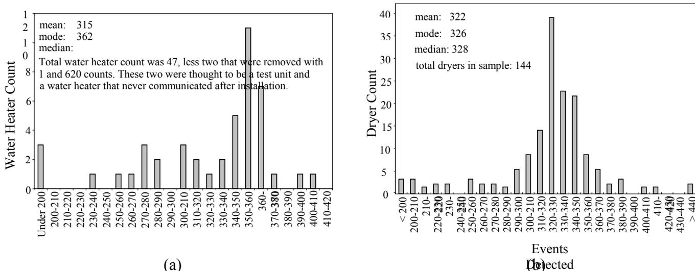
**Figure 4.** Distribution of Underfrequency Events Observed by Project (a) Water Heaters and (b) Dryers
