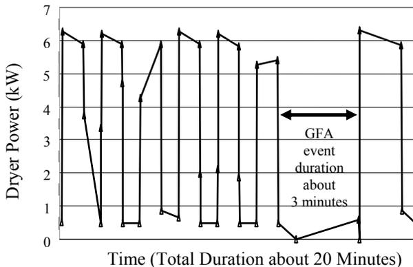
**Figure 5.** Response of a Single Project Clothes Dryer During a 3-Minute Underfrequency Event
