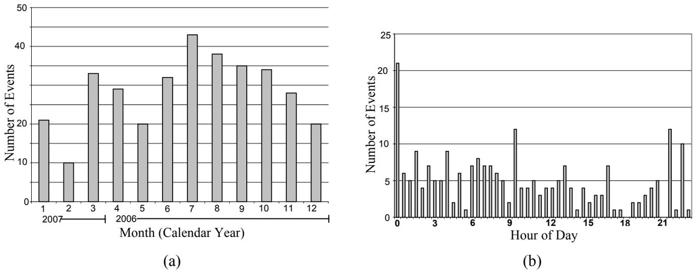
**Figure 8.** Total Underfrequency Events Recorded by the Project by (a) Month and (b) Hour
