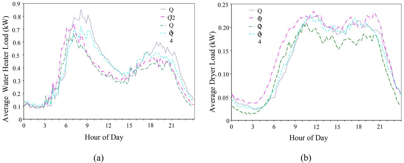
**Figure 9.** Average Daily Load Curves for the Project's (a) Water Heaters and (b) Clothes Dryers
