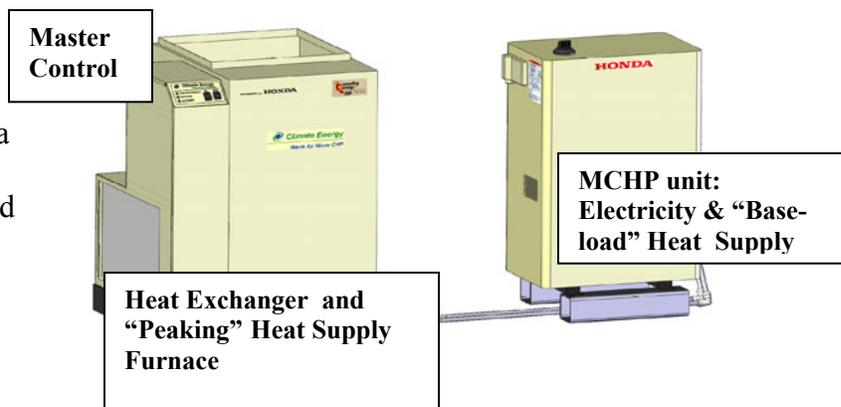
byproduct of the normal operation of the home. The engine provides approximately 11,000 btus per hour of thermal energy to the furnace. Simultaneously, the generator produces 1.2 kilowatts (kW) of electric power for the home. It is this process that maximizes the fuel to produce electric power and produce heat to satisfy the heating demand. The condensing furnace augments the 11,000 btus with the additional heat necessary to reach the homeowner's desired temperature.
