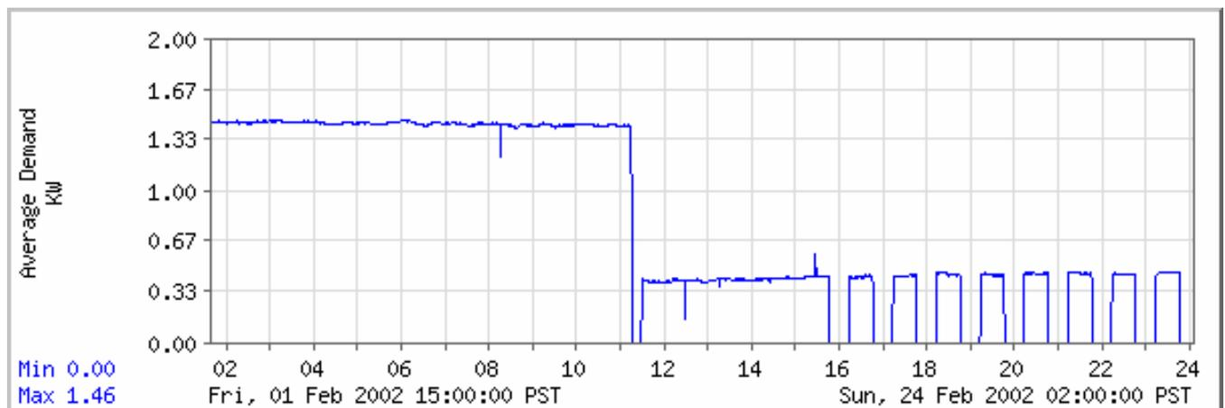
The graph above shows the kW consumption on one of several identical circuits. The data was gathered using an electrical meter installed in an electrical panel serving the
