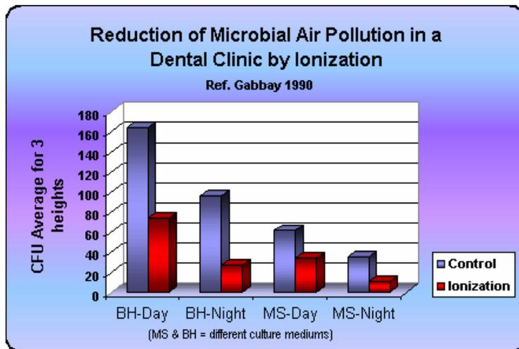
*This chart in figure 6 was presented by the Penn State Department of Architectural Engineering paper on Negative Air Ionization. It demonstrates the levels of colony forming units (CFU) in a dental clinic with and without ionization. Airborne ionization levels were reduced by 32-52% with ionization. The study was performed by Gabby, J. "Effect of ionization on microbial air pollution in the dental clinic" (1990)*
