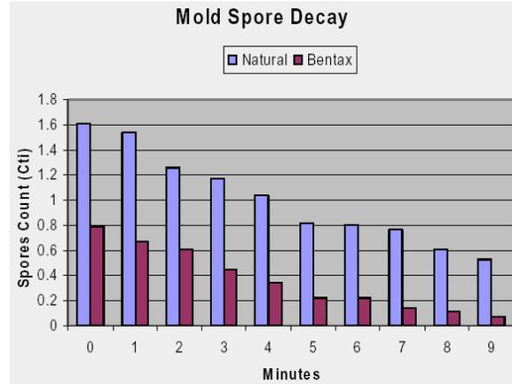
The graphs in figures 3 and 4 were excerpts of laboratory testing performed on bi-polar ionization equipment by Intertek ETL Semko. The tests show enhanced particle decay effect under ionized conditions.
