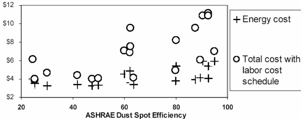
Figure 4. Monthly cost per 1000 ft<sup>3</sup> /min (470 L/s) of supply air for filters with different ASHRAE Dust Spot Efficiency ratings. Total costs include the costs of the filters, labor to remove and replace the filters, and fan energy.
