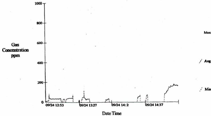
*The Graphs in figure 5 were taken from a field analysis of an industrial bi-polar ionization system used to control ethanol exhaust emissions. The analysis was performed by CTP Air Pollution Control in it's Report of Bentax VOC Reduction System at Scandiflex/Lanskinoo Rittsteig, K.*
