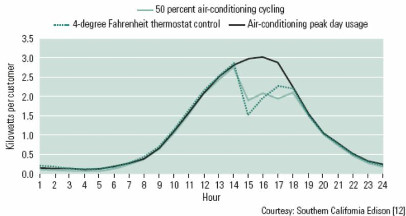
Because temperature offset produces most of its load reduction during the first hour, it's a good strategy for short events such as brief transmission constraints or local distribution problems. If the utility is running short events, it can do temperature offsets much more frequently than duty cycling because, overall, the customers won't be affected for as long. That's an attractive attribute for utilities wanting to use load control to alleviate relatively short-lived problems.
