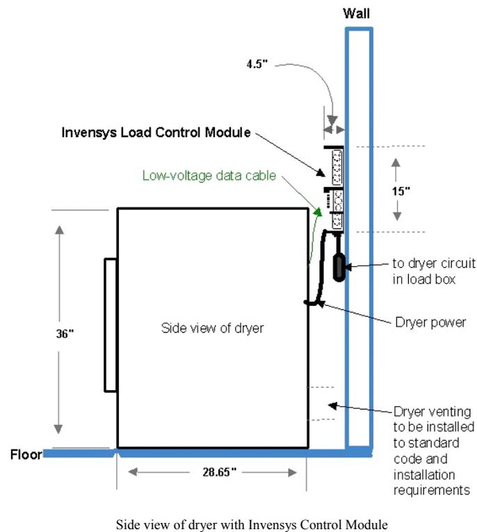
**Figure 4. Configuration of Dryer, Load Control Module and GFA Controller**
