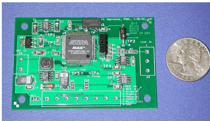
Figure 1. Grid Friendly Controller Produced for the Project
