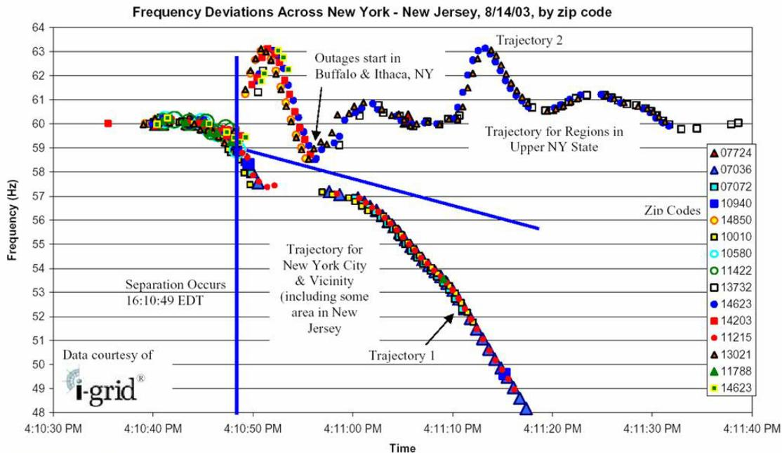
Figure 2. Power Grid Frequency Deviations During the August 2003 Blackout, by Zip Code
