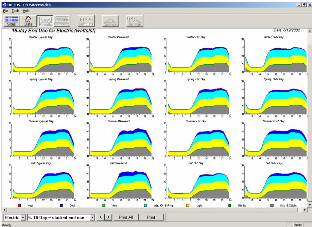
Figure 3: DrCEUS Results - 16-Day Hourly Electric End-Use (watts/sf)
