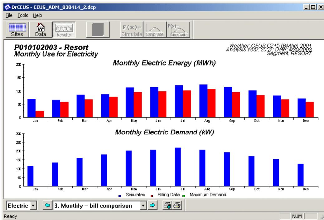
Figure 4: DrCEUS Results - Actual Billing versus Simulation
