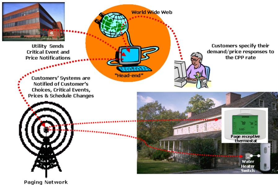
**Figure 1 - Simple One-Way CPP Configuration**
